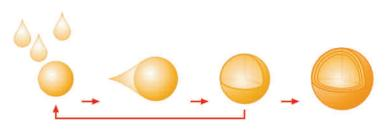
Spray granulation enables the drying of liquids while simultaneously forming dust-free granules.
