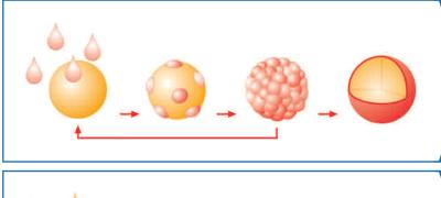
Spray coating covers particles with grain sizes from 100 microns to 3 millimeters with a defined layer in order to protect active ingredients or to functionalise particle surfaces.
