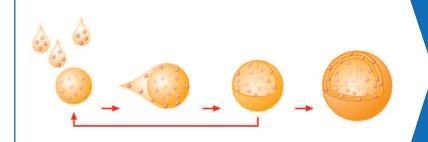
Spray encapsulation watery or hot-melt: Spray encapsulation helps to embed sensitive substances with homogenous distribution in a compact protection matrix.
